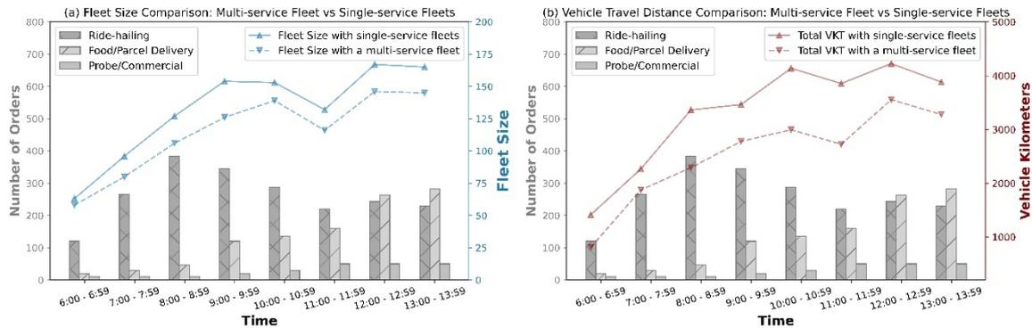
Figure 3 – Comparison of Minimum Fleet Size and Vehicle Kilometers
