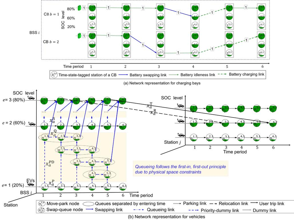
Figure 2 – Illustration of two time-electricity-expanded networks for charging bays and vehicles
