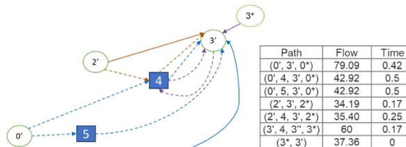
Figure 2. Recharge network and flow for recharging and rebalancing
